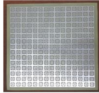
Fig. 9. The fabricated prototype of the proposed UWB FSS.
