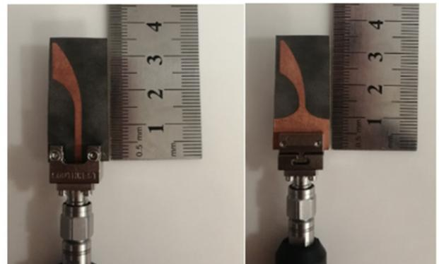
Fig. 10. The fabricated antenna design.
