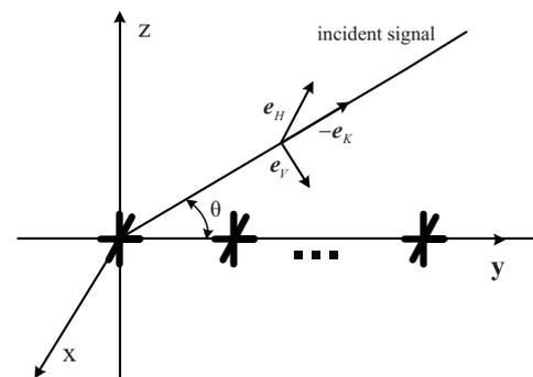
Fig. 1. The tri-polarized nested array.
