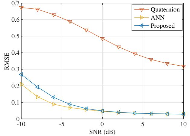
Fig. 6. RMSE of DOP estimation under different SNRs.
