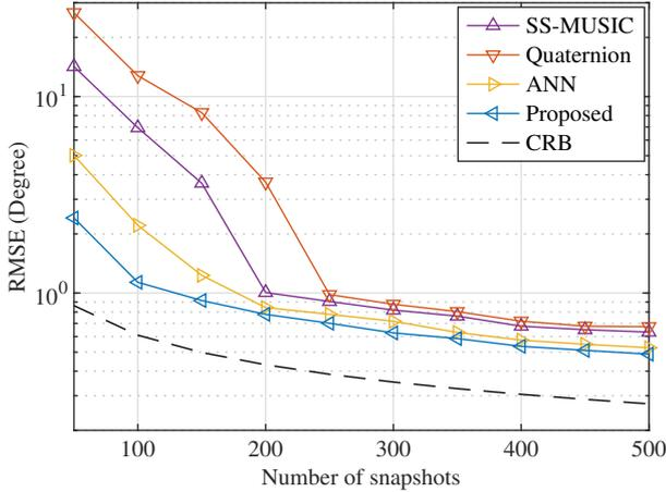
Fig. 5. RMSE of DOA estimation under different number of snapshots.
