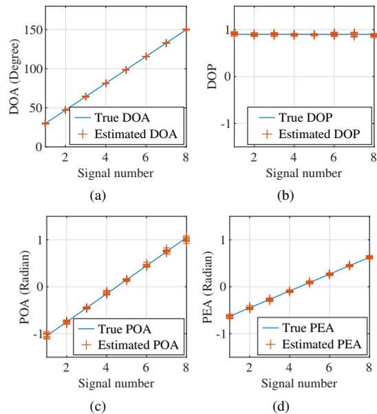
Fig. 3. The estimated DOAs and polarization parameters of ten trials: (a) DOA, (b) DOP, (c) POA, (d) PEA.
