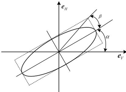
Fig. 2. The polarization ellipse.
