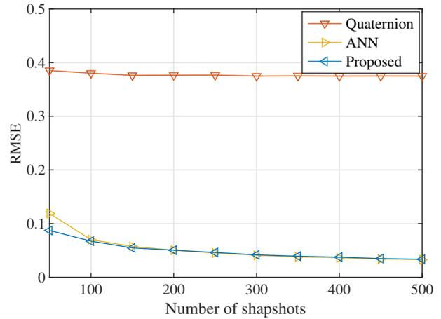
Fig. 7. RMSE of DOP estimation under different number of snapshots.
