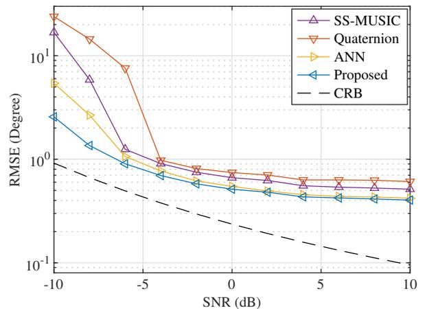
Fig. 4. RMSE of DOA estimation under different SNRs.
