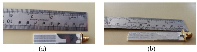
Fig. 16. Fabricated antenna: (a) top view, (b) side view.
