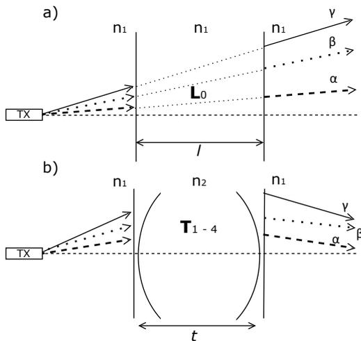
Fig. 4. Three different deflected optical beams propagate a) in a medium with a constant refractive index  $L_0$  and b) a medium with a thick lens  $T_{1-4}$ .  $\alpha, \beta,$  and  $\gamma$  indicate specific optical beam deflections in each model.
