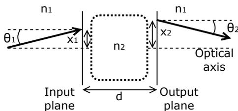
**Fig. 1.** The optical beam transmission technique, where  $x_{1,2}$  represent the deflections of the beam from the optical axis,  $\theta_{1,2}$  indicate the angles of deflection and  $d$  is the distance between the input and output planes.
