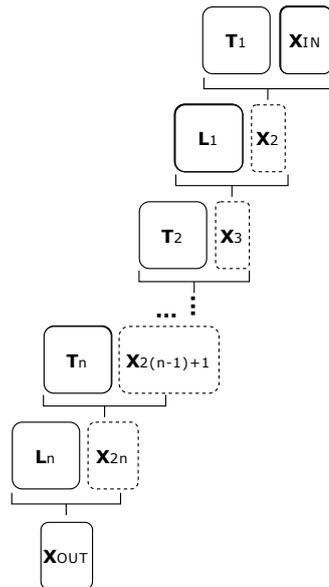
**Fig. 9.** Diagram showing the procedure of cascade matrix calculation. The bold blocks represent the input deflection vector, the ABCD matrices, and the output deflection vector. Dashed blocks indicate deflection vectors by passing through the individual elements of cascade.
