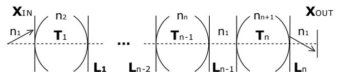
Fig. 8. Illustration model of the cascade of  $N$  turbulent cells.
