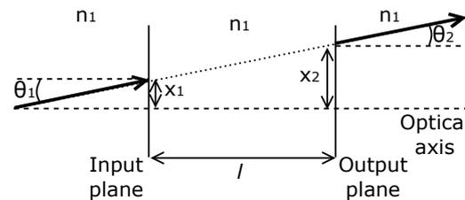
**Fig. 3.** Beam propagation through a medium with a constant refractive index, where  $l$  denotes the distance between the input and output planes and the equality of angles applies  $\theta_1 = \theta_2$ .
