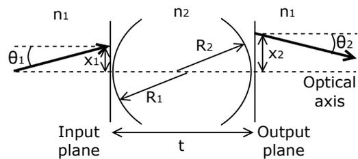
**Fig. 2.** Beam propagation model through a thick lens, where  $t$  denotes the center thickness of the lens, which also represents the distance between the input and output planes.  $R_{1,2}$  are the radii of curvature of the lens surfaces [18].
