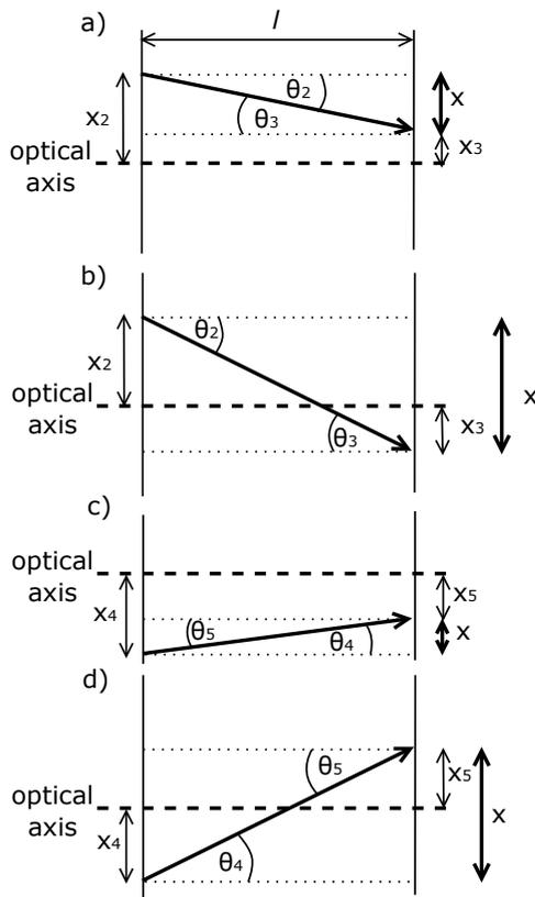
Fig. 7. Four cases of the laser beam transition from the space below and above the optical axis of the system. a) and b) represent the area  $L_1$  in Fig. 6, and c) and d) represent the  $L_2$  region in the same figure.
