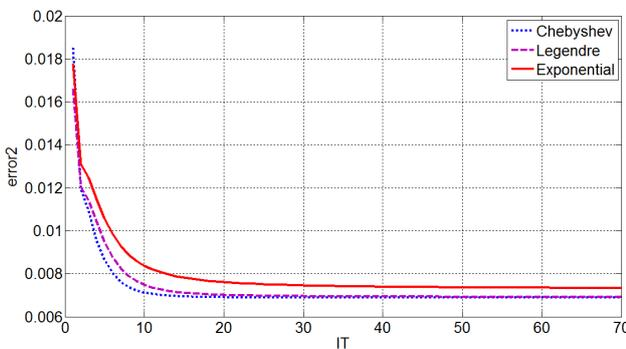
Fig. 10. Defined error2 versus total number of iterations,  $IT$  for Taylor excitation.
