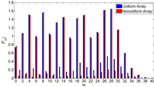
Fig. 14. Magnitude of orthogonal coefficients of Chebyshev polynomials for raised linear excitation.
