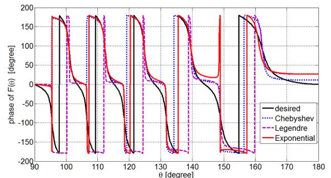
Fig. 13. Phase of the array factors of NSAA designed by three OCE methods for raised linear excitation.
