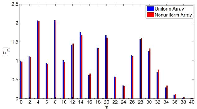
Fig. 7. Magnitude of orthogonal coefficients of Chebyshev polynomials for Chebyshev excitation of SLL =  $-20$  dB.
