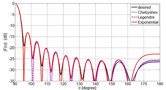
Fig. 12. Magnitude of the array factors of NSAA designed by three OCE methods for raised linear excitation.
