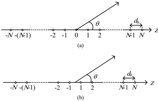
Fig. 1. Typical configuration of USAA: a) Odd number of elements. b) Even number of elements.
