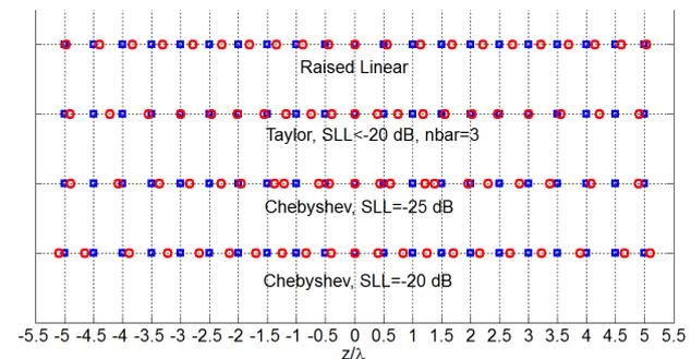
Fig. 19. Positions of USSAs and NSAAs obtained by Chebyshev polynomials.  $\square$ : USSA.  $\circ$ : NSAA.
