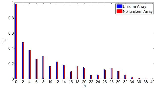
Fig. 8. Magnitude of orthogonal coefficients of Legendre polynomials for Chebyshev excitation of SLL = -20 dB.
