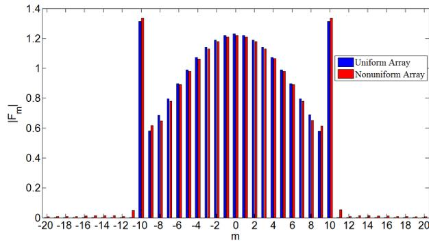
Fig. 9. Magnitude of orthogonal coefficients of Exponential functions for Chebyshev excitation of SLL = -20 dB.
