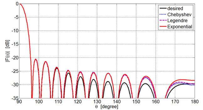
Fig. 11. Array factors of NSAA designed by three OCE methods for Taylor excitation of SLL < -20 dB.
