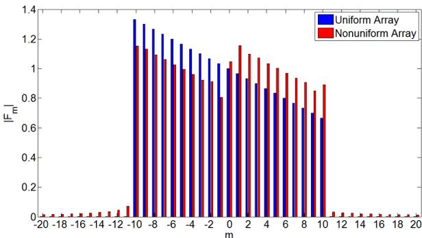
Fig. 16. Magnitude of orthogonal coefficients of Exponential functions for raised linear excitation.
