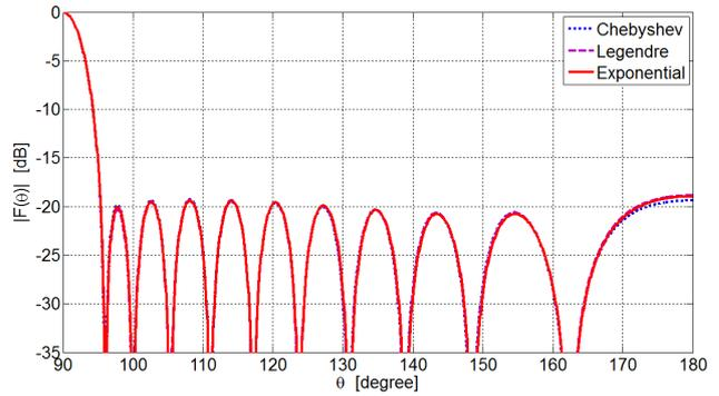
Fig. 5. Array factors of NSAA designed by three OCE methods for Chebyshev excitation of SLL =  $-20$  dB.
