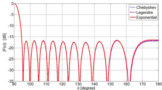
Fig. 4. Array factors of NSAA designed by three OCE methods for Chebyshev excitation of SLL =  $-17$  dB.
