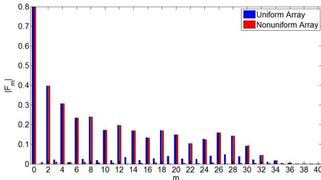
Fig. 15. Magnitude of orthogonal coefficients of Legendre polynomials for raised linear excitation.
