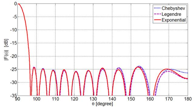
Fig. 6. Array factors of NSAA designed by three OCE methods for Chebyshev excitation of SLL =  $-25$  dB.
