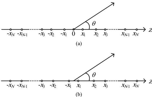
Fig. 2. Typical configuration of NSAA: a) Odd number of elements. b) Even number of elements.
