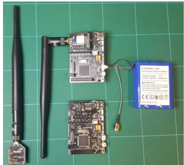
Fig. 4. LoRa and BLE modules with Wasmote PRO v1.5.
