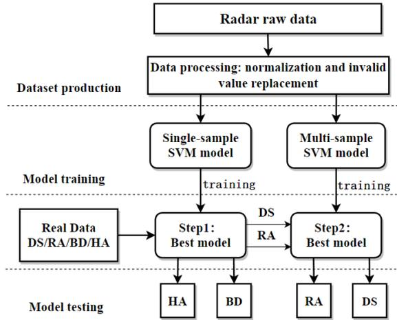
Fig. 9. The structure of four kinds of target hydrometeor classification system model.
