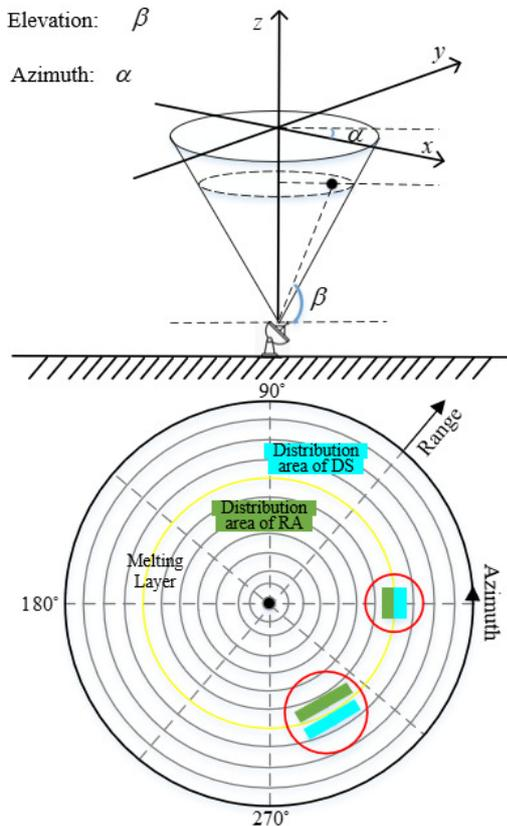
Fig. 5. PPI scanning mode of dual polarization radar and the different fusion methods in this scanning mode.
