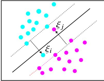
Fig. 1. Two-dimension SVM model with slack variables.
