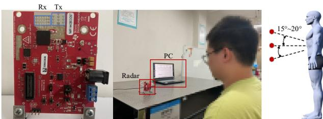
Fig. 8. (a) is the experimental environment, (b) is IWR 1443 Boost radar and (c) is the radar measurement angle diagram.
