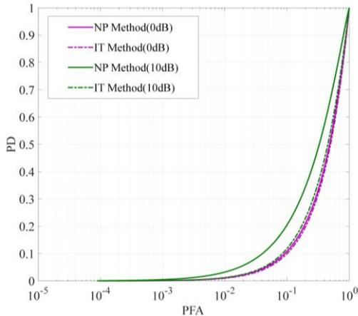
Fig. 5. The ROC for the IT detection method and the NP detection method.
