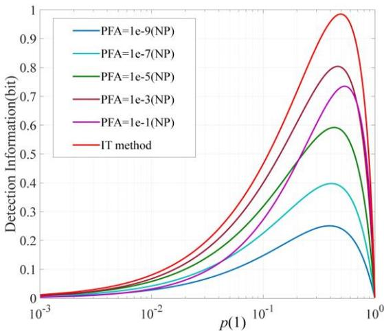
Fig. 3. The relationship between detection information and target existence probability.
