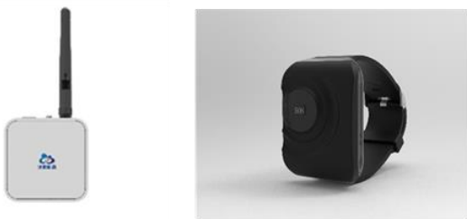
Fig. 5. Experimental data collection setup: UWB localization base station (left) and TOA positioning tag (right).
